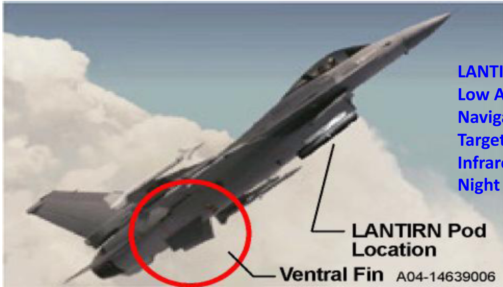
Figure 1. LANTIRN pod carriage on the F-16.
